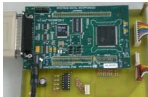
Figure 9. TMS320F2812 eZdsp board for controller realization
