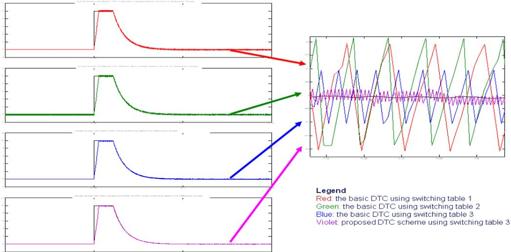
Fig. 7. Comparison of the electromagnetic torque response under the basic DTC using eight-state table, using six-state table, using bipolar torque eight-state table, and under proposed DTC scheme
