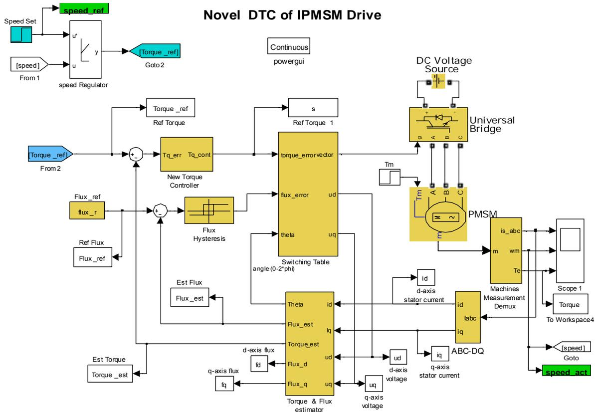
Fig. 6. A block diagram of a proposed DTC system for PMSM drives
