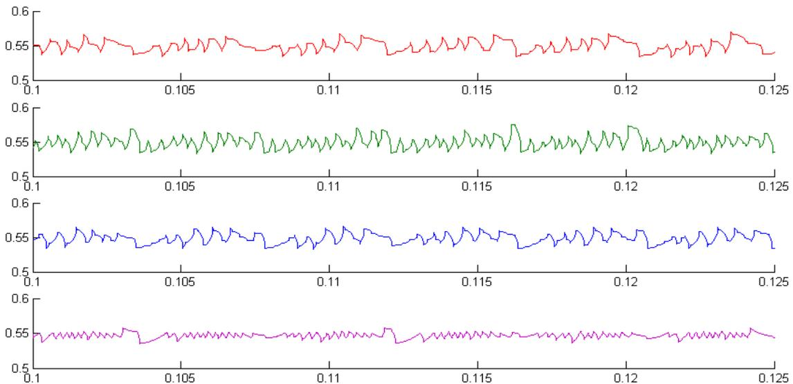
Fig.8. Comparison of the flux response under the basic DTC using eight-state table, using six-state table, using bipolar torque eight-state table, and under proposed DTC scheme
