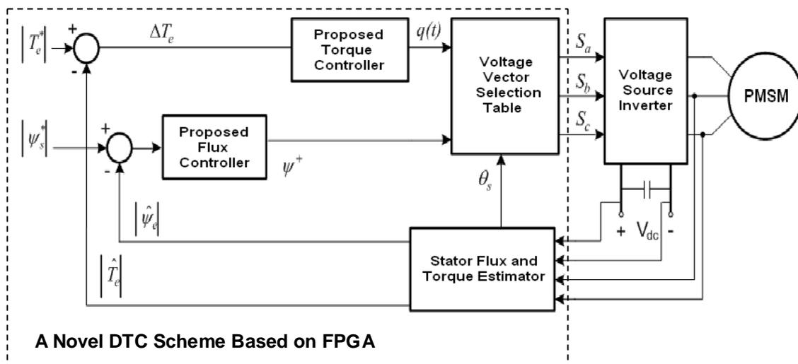
Fig 4. Block diagram of proposed a novel DTC scheme of PMSM drive using FPGA
