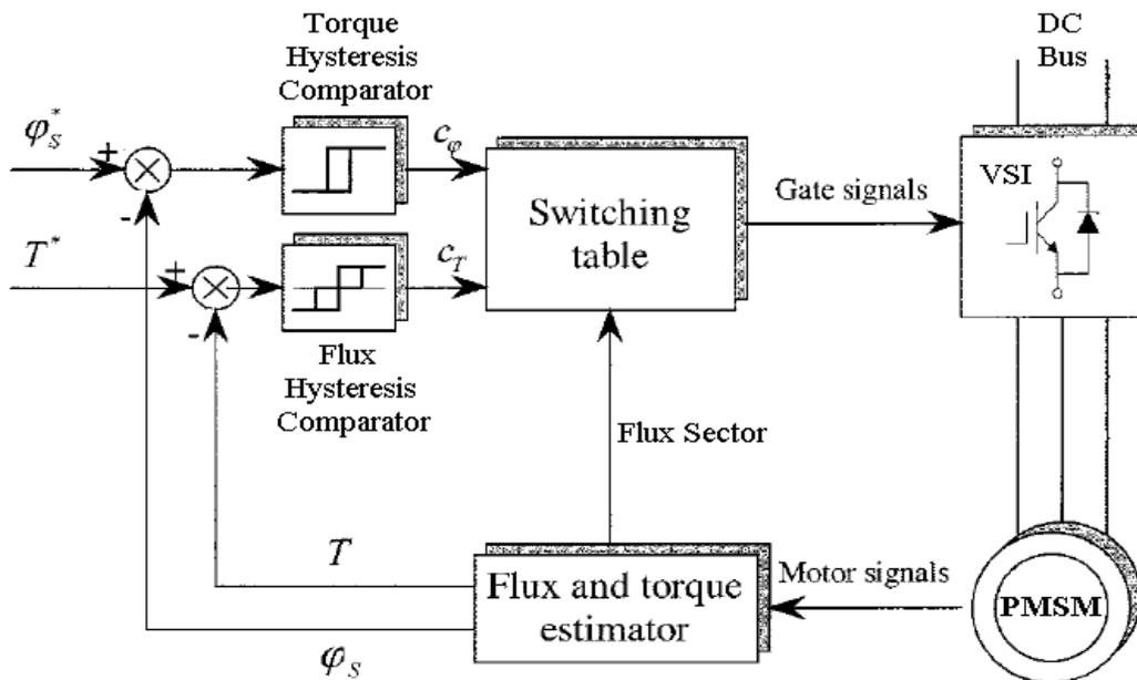
Fig. 3. Basic DTC scheme of PMSM drive system.
