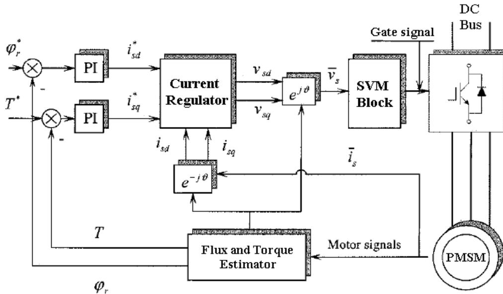
Fig. 2. Basic FOC scheme of PMSM drive system.
