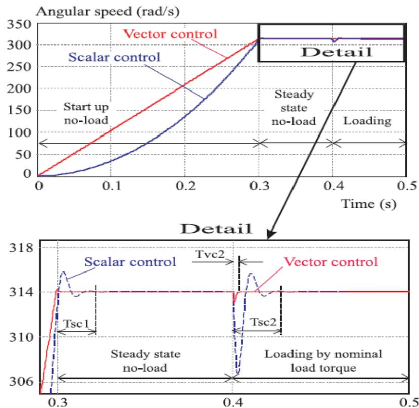
Fig. 1. Angular speed of PMSM controlled by Vector control and Scalar control strategies.
